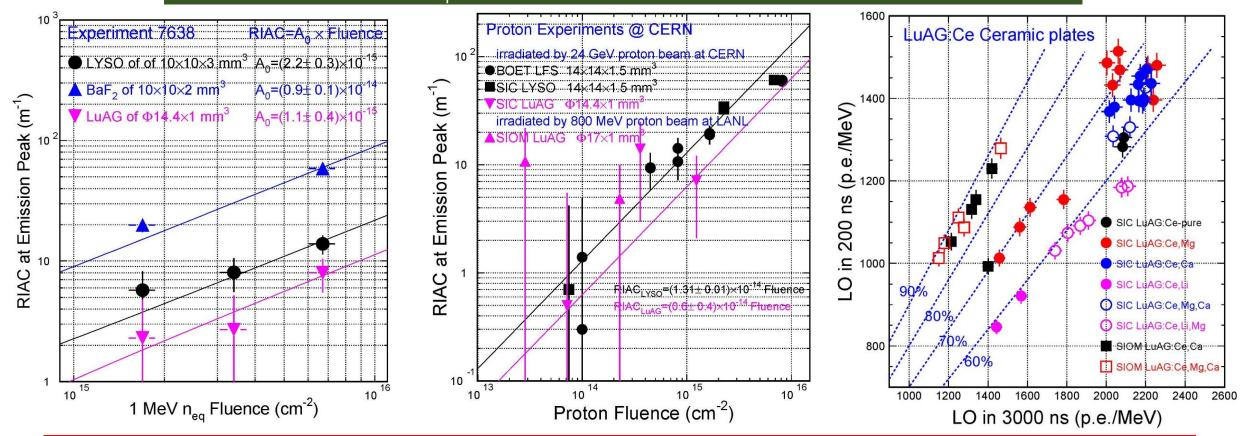
R&D on slow component suppression by Ca co-doping, and radiation hardness by  $\gamma/p/n$
