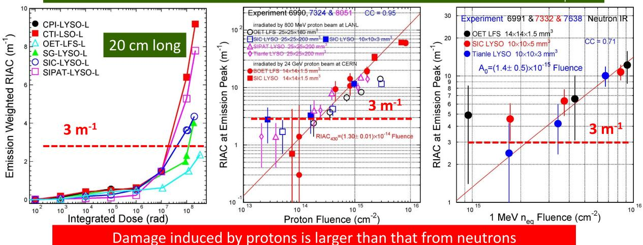
Due to ionization energy loss in addition to displacement and nuclear breakup
