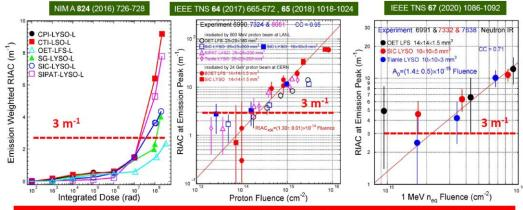
Crystals damaged by both proton and neutron. Damage by proton is larger than that from neutrons because of ionization energy loss in addition to displacement and nuclear breakup
