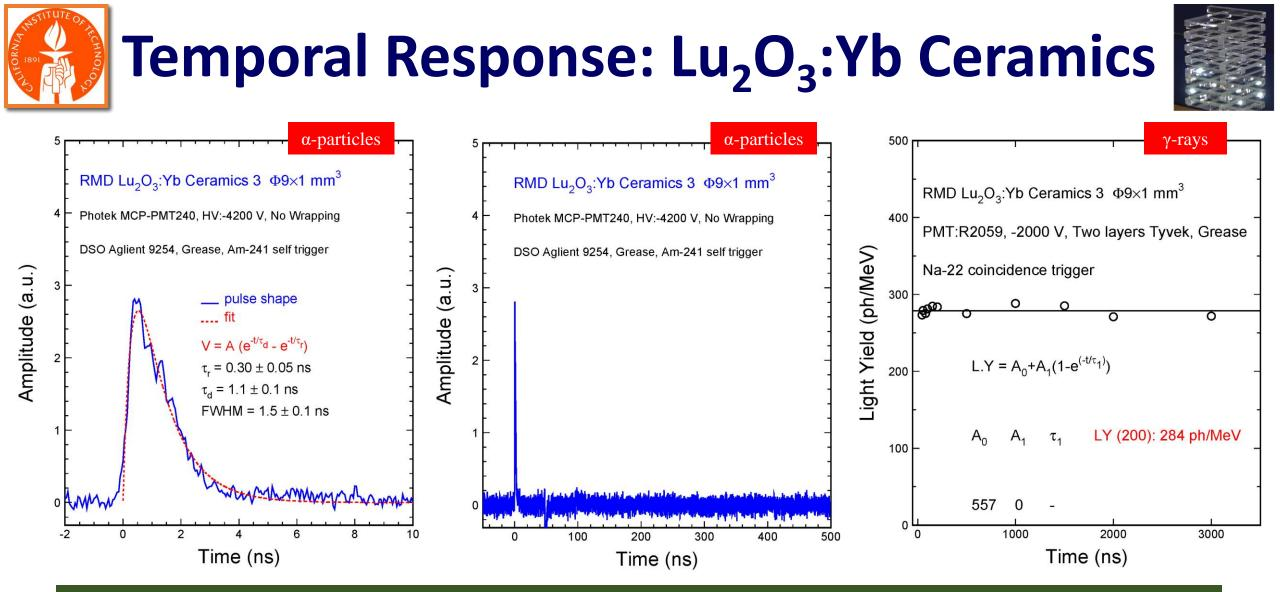
$Lu_2O_3$ : Yb ceramic of 9.4 g/cc shows an ultrafast decay time of **1.1 ns** by Am-241 with negligible slow component observed in integrated light output measurement
