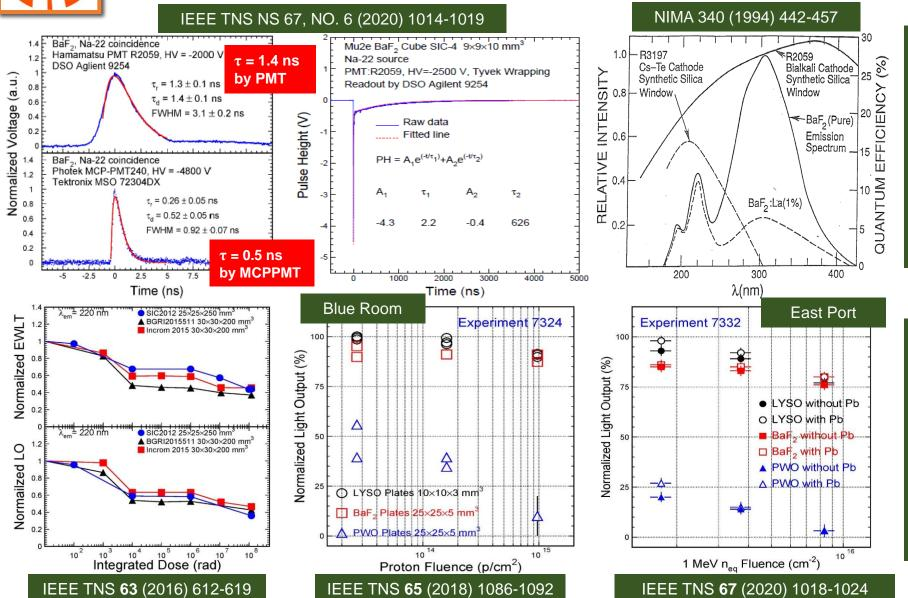
$BaF_2$  has an ultrafast scintillation component @ 220 nm with 0.5 ns decay time and a much larger slow component @ 300 nm with 600 ns decay time.
