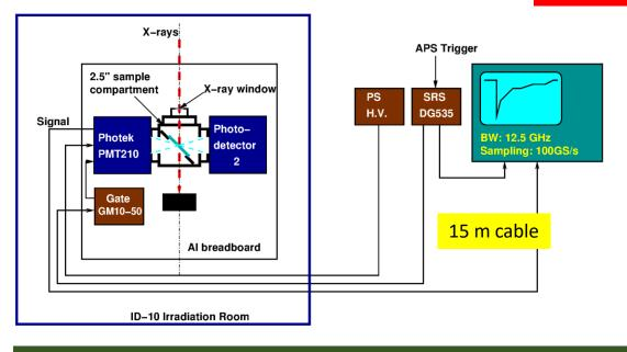
The decay time of BaF<sub>2</sub> measured at APS for septuplet X-ray bunches with 2.83 ns spacing is longer than 1 ns. This is suspected to be caused by the 15 m long cable used between the MCP-PMT and the MSO
