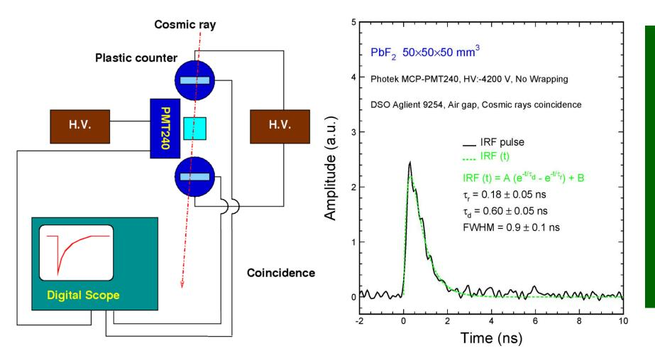
Intrinsic ultrafast response time can be extracted by taking out the IRF of the setup. It was measured by fitting Cerenkov light pulse from a PbF<sub>2</sub> crystal, which agrees well with Photek spec.
