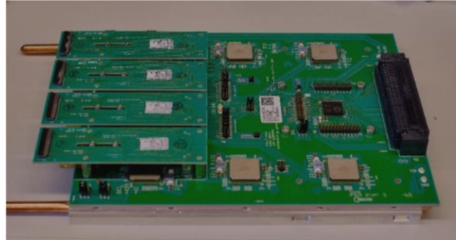
Data and Control Board
