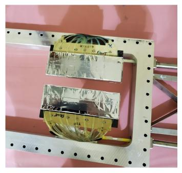
Fibers were light tightened with a thin tedlar sheet.
