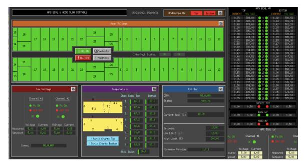
Last run we had cooling issues, affected by underperforming chiller and high ambient temperatures in alcove. Mitigated by forced air from duct from AC into alcove, and better ECAL insulation, need to resurrect those mitigations. Chillers were tested/serviced.
