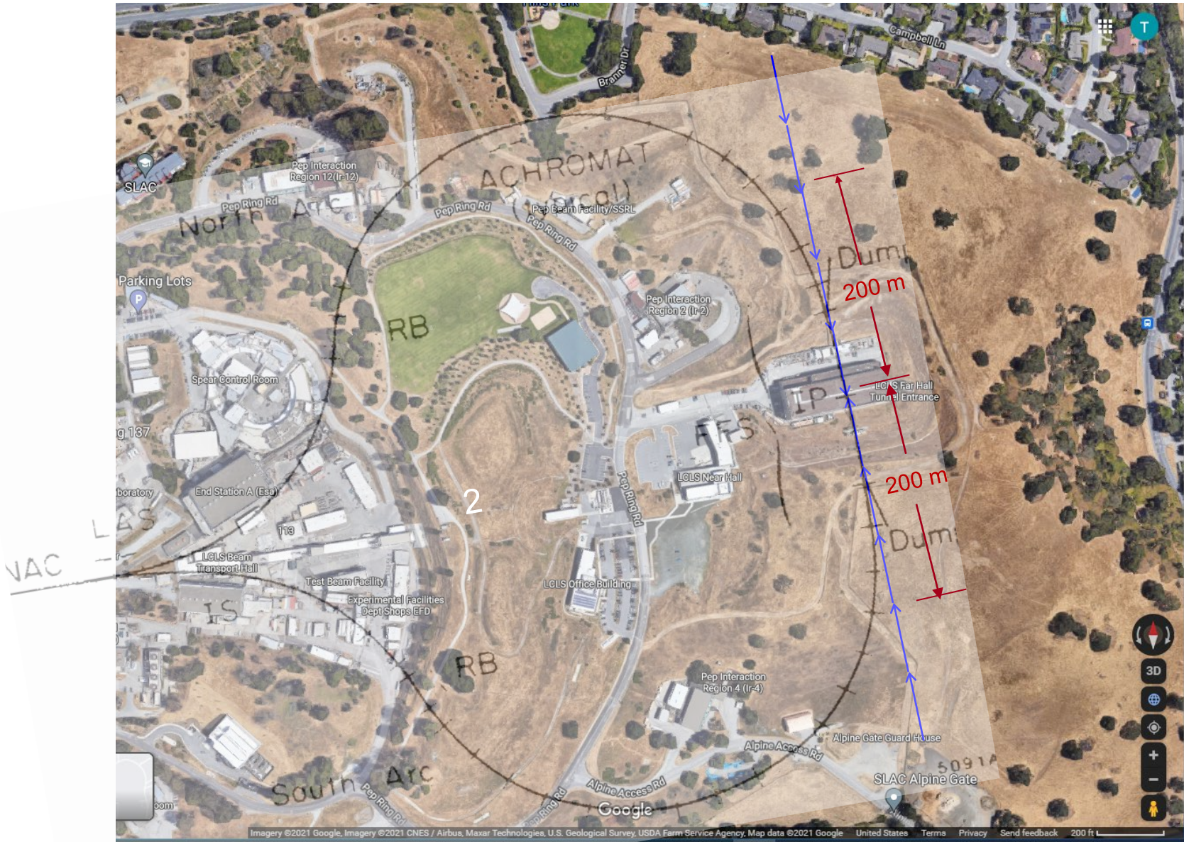
SLC FF straight sections are each about 100 m long.
