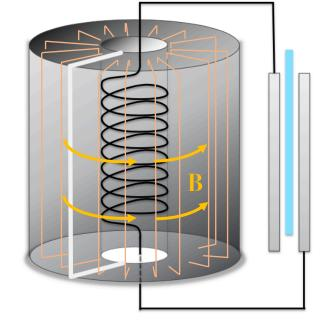
To shield resonator from losses → make "snake swallowing its own tail" geometry
