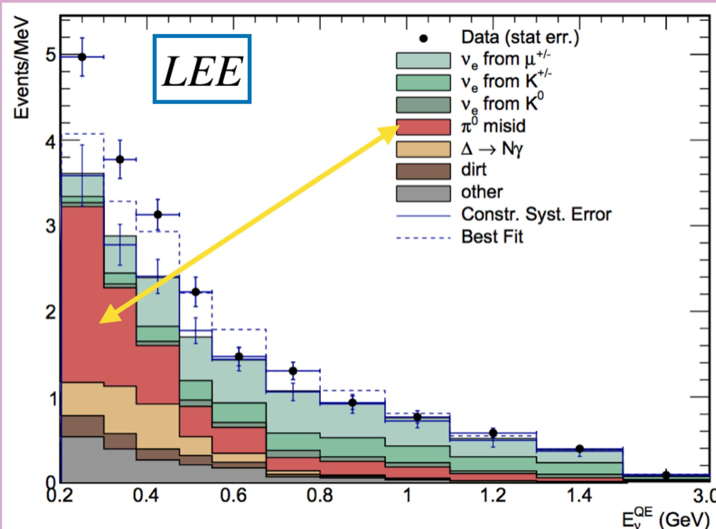
MiniBooNE  $\nu_e$  measurement shows a significant excess of  $\nu_e$ -like interactions below 500MeV (Low Energy Excess) with:
