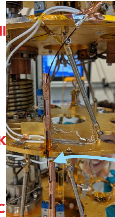
Twisted Pair NbTi (CuNi) Magnet Wire (Thermalized to plates.)
