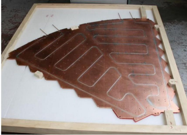
Fig. 6. CE-E copper cooling plate prototype
