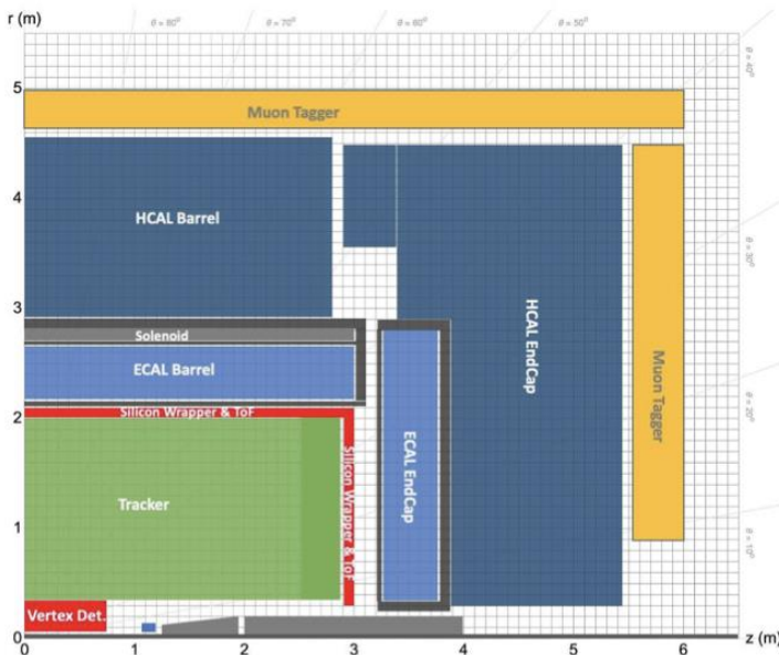
Figure 1. Sketch of a cross-section of a quarter of the ALLEGRO detector concept (left) and 3D view of the implementation into the FCC-SW (right).
