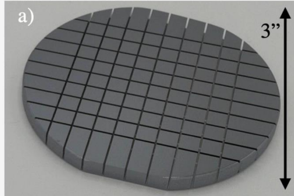
KID array on the other side of the wafer hosting 60 resonators (60 nm Al)
