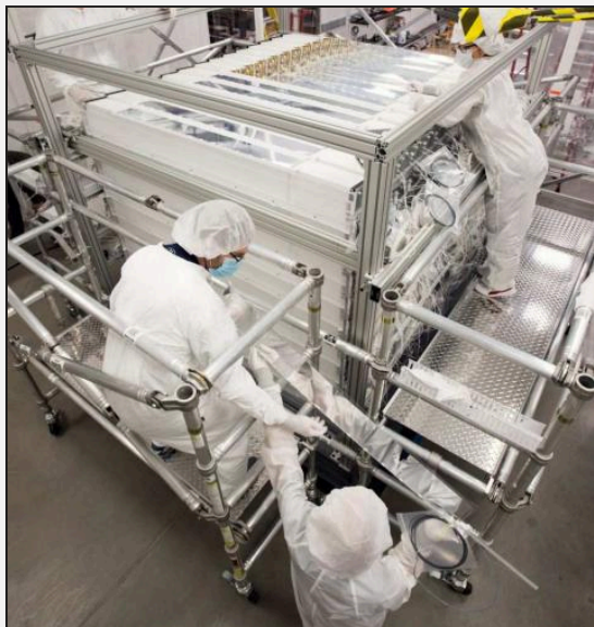
PROSPECT — segmented liquid scintillator at HFIR; a tonne of detector under assembly.
