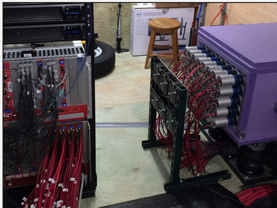
miniCHANDLER — 80 kg of solid scintillator in a trailer, operating at a reactor at room temperature.
