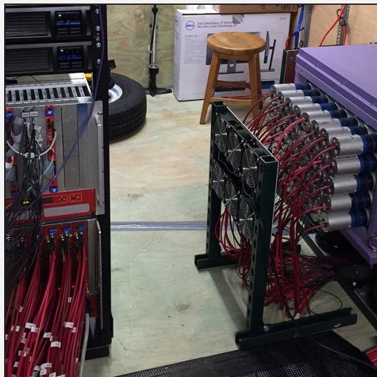
miniCHANDLER — a mobile solid-scintillator demonstrator, plus the rack of electronics that goes with it.
