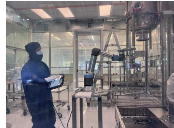
Cobot-assisted cavity assembly for vertical test
