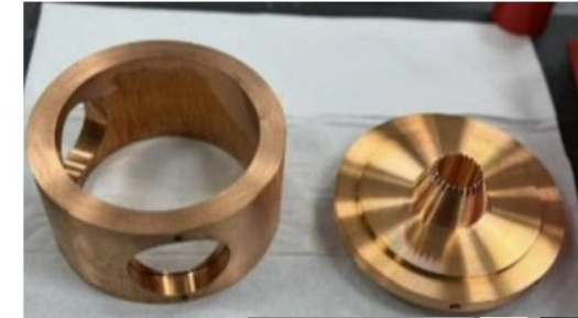
Cavity 3- output cavity assembly
