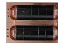
REBCO coated conductor cavity for Axion, T. Puig
