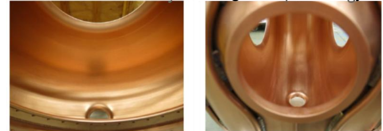
Mirro-like surface finishing in MICE cavity
