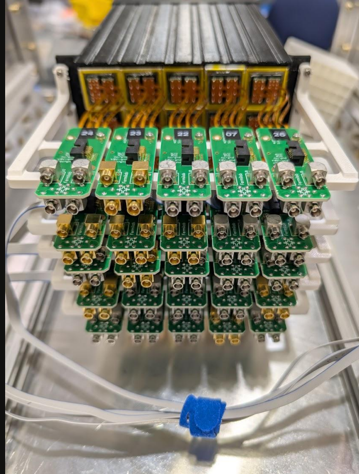
Rear matrix with new FNAL amplifiers
