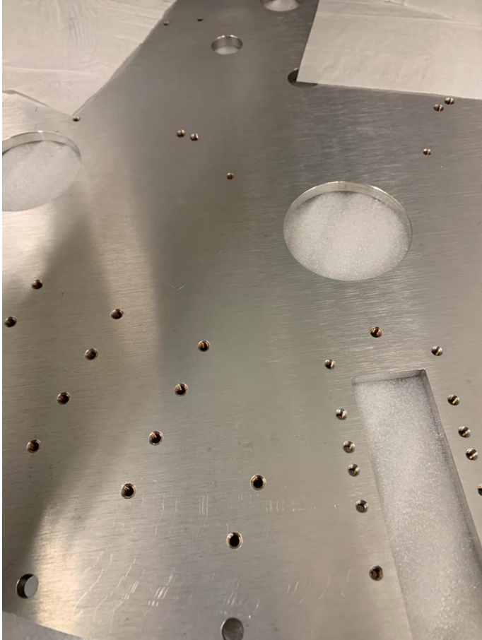
PhBr helicoils installed
