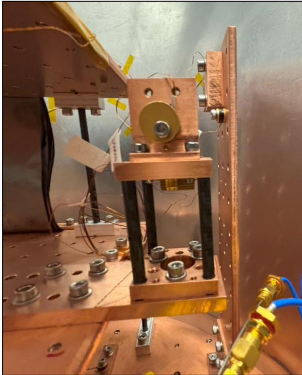
Variable temperature stage for noise calibration
