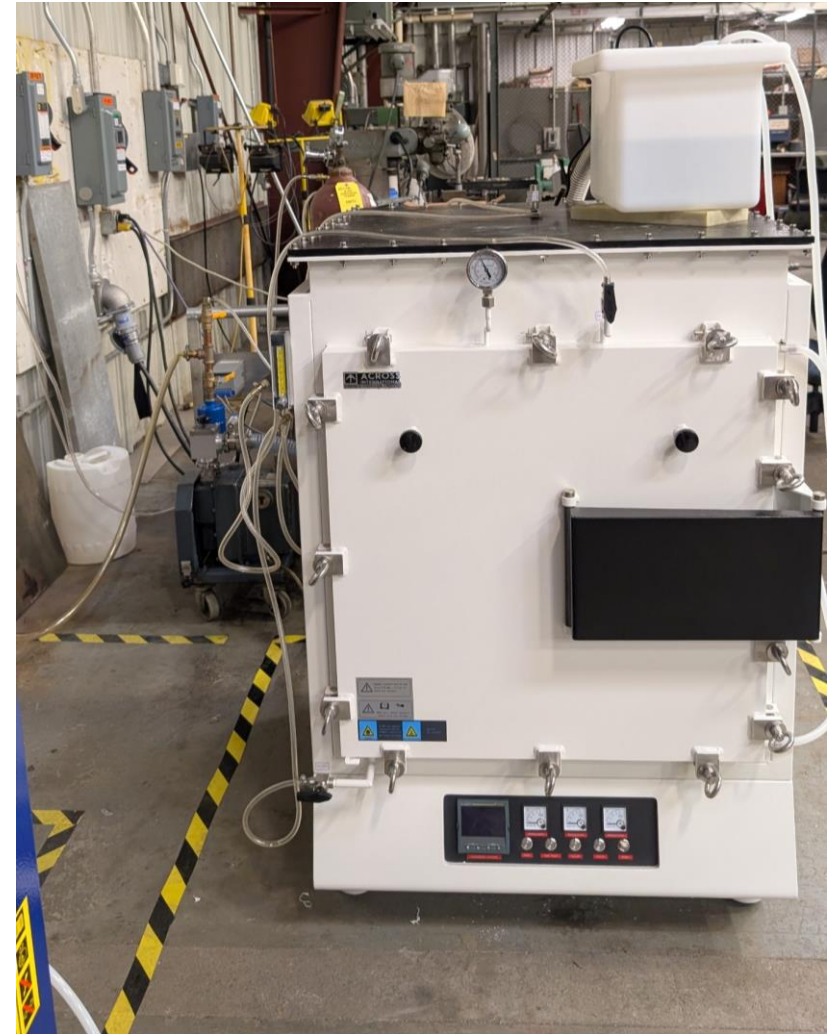
Furnace for heat treatment
