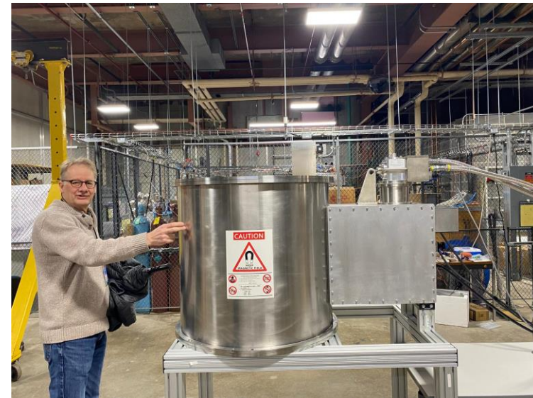
7.5 T, 30 cm bore conduction-cooled magnet for HTS tape inspection- commissioned last April
